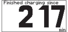
The battery symbol indicates the current state of charge. The greater the number of bars that are displayed, the further advanced the charging process is. As soon as the battery is fully charged, a minute counter will appear (see figure on right). This counts the minutes since the end of charging; when a number of chargers are being used, this makes it easier to decide which battery will have already cooled down most.
