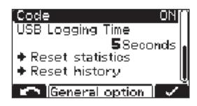
Time interval (s) for recording charging parameters on the USB flash drive (USB Logging Time)
