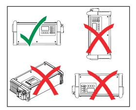
The permissible operating position of the device is horizontal.
