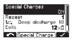
Selecting "Special Charges" allows one or more of the alternative charging types to be performed temporarily:
