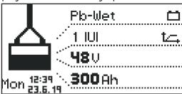
In standard mode, the display shows the following charger parameters:
