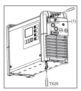
The cover (1) for the USB port can be secured with a screw.
