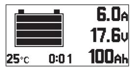
When the battery is fully charged all 4 bars of the battery symbol appear black. As soon as the battery is fully charged, the charger begins conservation charging.
