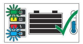
For an optimal battery life, only disconnect the battery from the battery charger when the blue "Battery cooled down" indicator is showing in addition to the green indicator, in accordance with the explanation below. If several battery chargers are in use, first disconnect the battery which has been fully charged for the longest (the coolest).
