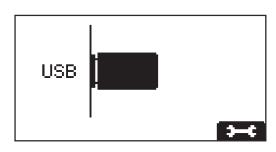
In USB mode, the display shows whether or not a USB flash drive is connected.
