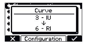
If the setting is not confirmed, the charger returns to configuration mode and the setting can be changed to the desired value.
