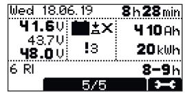
Use the "Up/Down" keys to switch between the pages for each stored charging process.
