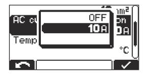
The minimum and maximum values differ depending on the different device classes. The minimum value is approx. 25% of the maximum nominal current of the charger.
