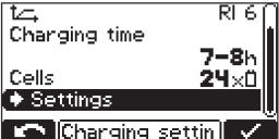
the display may vary depending on the selection made. If the "Pb-WET" type of battery has been selected in combination with the "RI" characteristic ("Curve") as in the example here, the "Ah" heading is replaced by the "Charging time" setting option.
